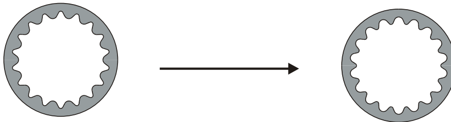
Figure 7: Effect of varying fin thickness for tubes having equivalent diameter
