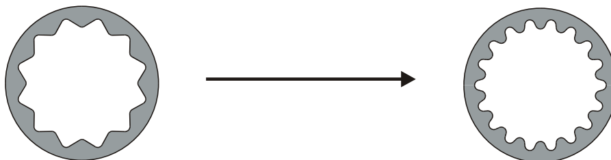
Figure 8: Varying fin number by changing trough radii for tubes having equivalent diameter
